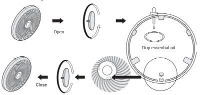
When assembling, first insert the large round hole according to the alignment mark, and then rotate clockwise
